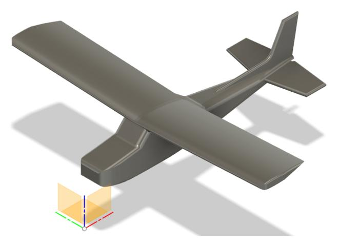
The wing span is just short of one meter and about 750mm nose to tip, so this needs to be chopped up in parts that will fit on my 3D print bed of  $230 \times 230 \times 250$ .
